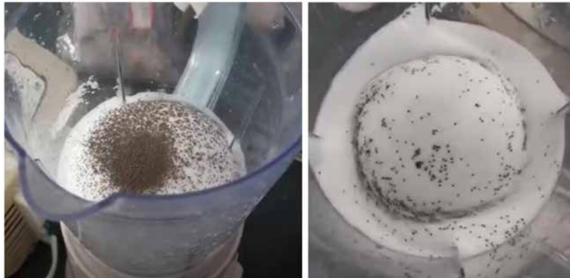
Figure 14—Proppant Suspension of the S-Gel CO 2 Foam in a Waring Blender
