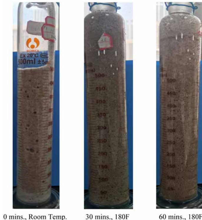
Figure 15—Sand Settling study of 10 gpt S-Gel CO 2 Foam at 180°F using 4 ppa of 40/70 Mesh Ceramic Proppant
